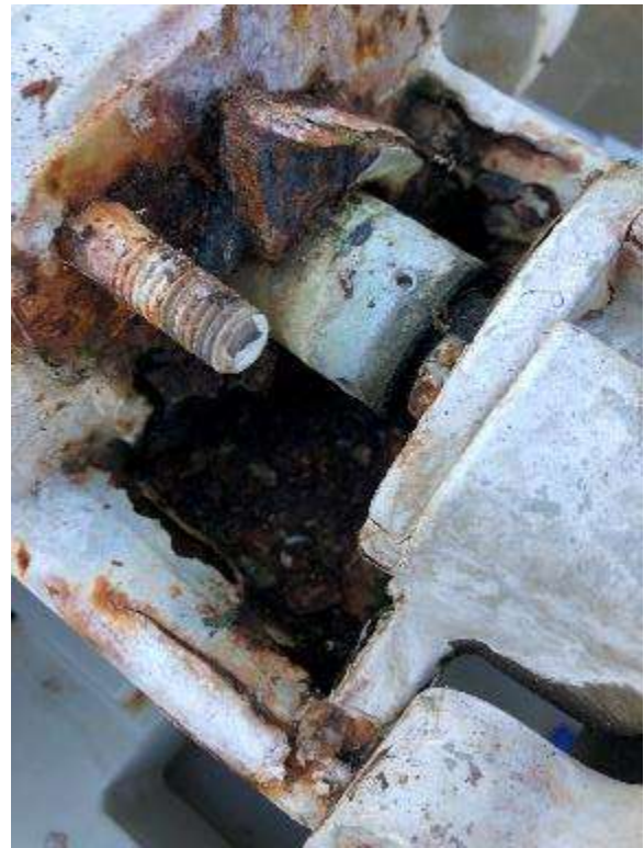
Packing flange corroded in half on UW Pump 1
