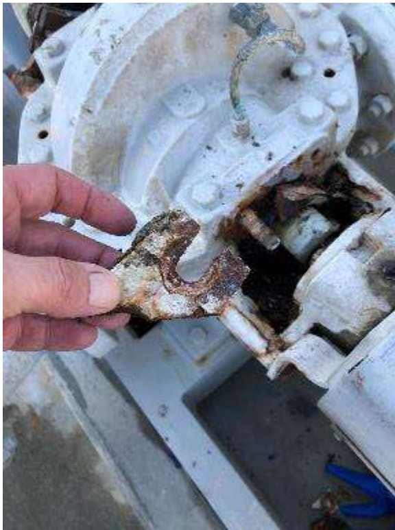
Packing flange corroded in half on UW Pump 1
