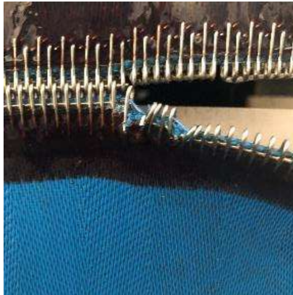
Broken Seam Wire on Belt Press Belt
